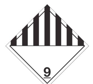
Use Class 9 Miscellaneous Dangerous Goods and UN Identification labels for transportation of lithium ion batteries which are assigned Class 9. Refer to relevant transportation documents. Lithium and lithium ion cells and batteries are regulated in the U.S. in accordance with Part 49 of the Code of Federal Regulations, (49 CFR Sections 105-180) of the U.S. Hazardous Materials Regulations.
